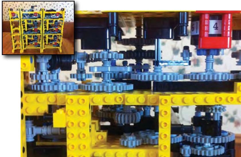
This picture shows some of the details of a Babbage Difference Machine designed and built by Andrew Carol. The inset shows the entire machine.
