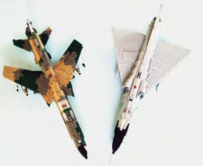
The F-105 (left) and F-106 (right) showing their swept wings and their area-ruled fuselages.
