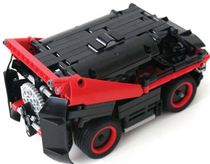
Another view of the A-Team's van, which shows the rounded IR control sensor. The large gear is attached to the drive motor, which is an XL motor.
