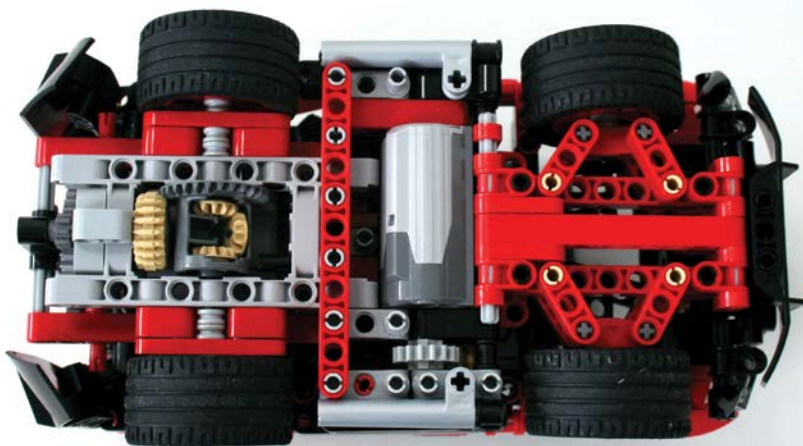
A look at the bottom of the van showing the differential gear for the drive. The M motor is actually the steering motor.
