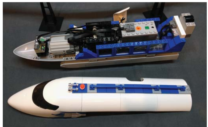
Monorail Blue's interior, showing the motor and battery within the body. The Power Functions receiver is at the rear of the model, making this a free-moving train.
