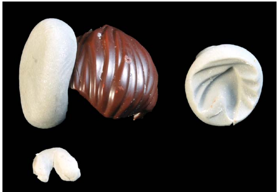
Top: Clay applied over hairpiece and prototype ear. Right: Mold made of ear and hairpiece. Bottom: Ear sculpt from clay.
