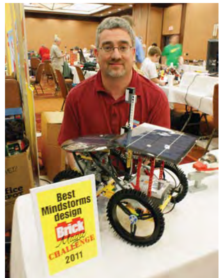
Sam Forker, above, built a rover that used a MINDSTORMS NXT and solar panels to power itself. He demonstrated it outside during the weekend.
