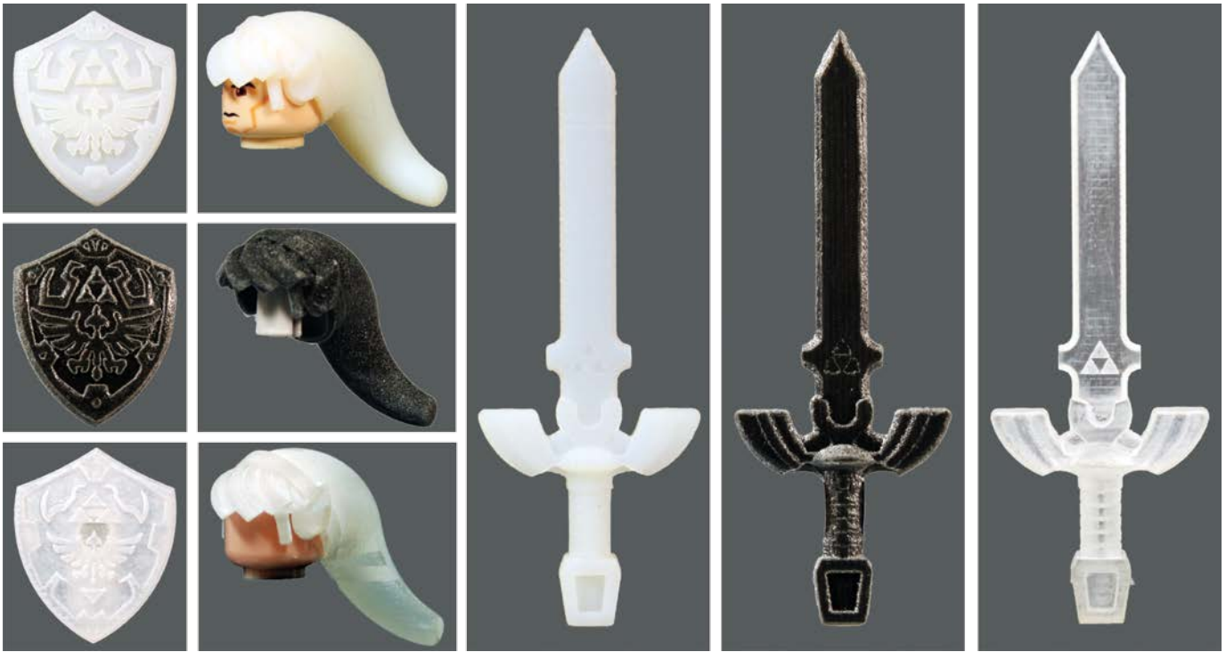
The same parts printed by Shapeways and Kraftwurx with various resolutions. Left two columns, top down, are as follows: White Strong and Flexible from Shapeways, Black Strong and Flexible from Shapeways, Nano Clear HD from Kraftwurx. The Swords from left to right are White Strong and Flexible, Black Strong and Flexible, and Nano Clear HD. Notice the print pattern on the Nano Clear sword. This can be removed with sanding, however, be careful not to remove your print detail or sand your part too thin. Note: the Shapeways shields (White Strong and Flexible and Black Strong and Flexible) are much larger than the Kraftwurx (Nano clear HD) print; for scale see the Multicolor Links or Shield figure.
