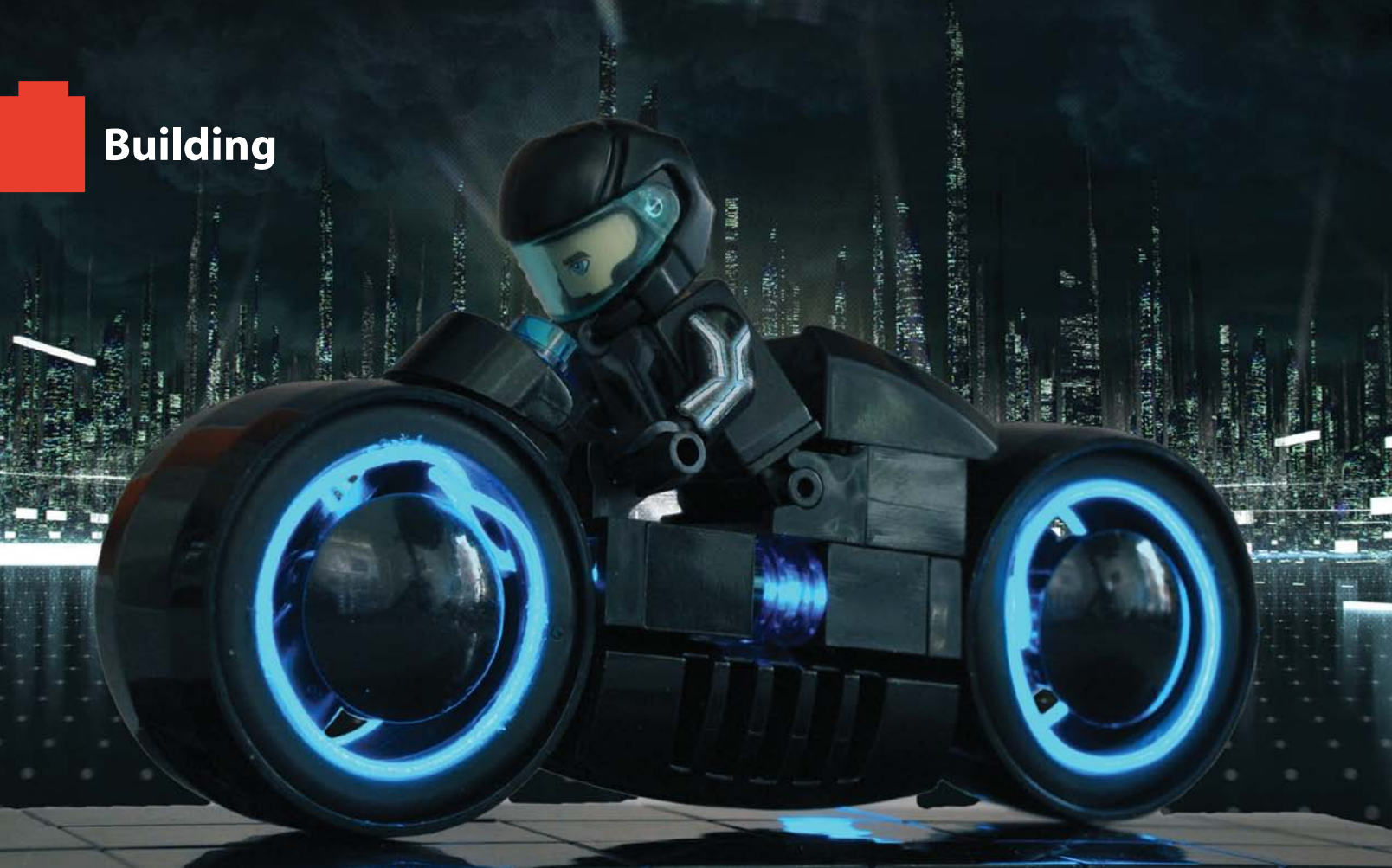
Figure 1: EL wire TRON Light Cycle, illuminated with 1.5 ft of EL wire and a 1 AA battery box/inverter.
